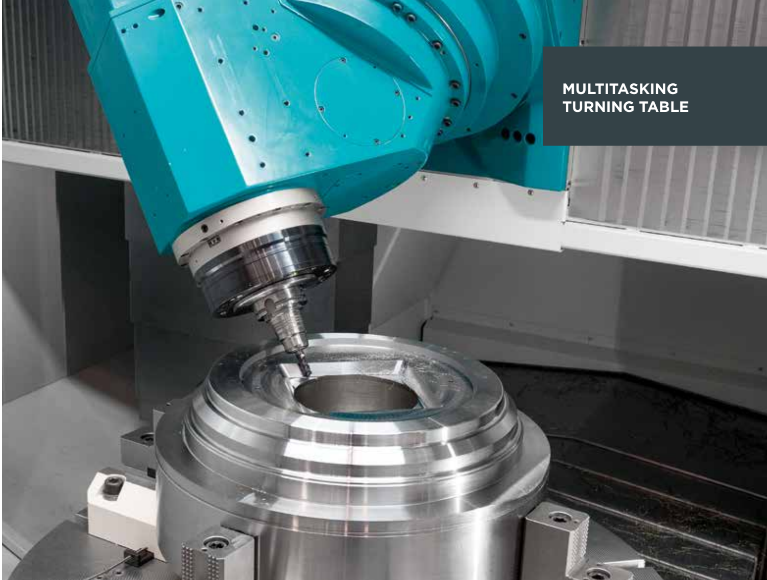
Milling and turning rotary table. Based on a combination of axial/radial bearing for turning and preloaded hydrostatic support for milling mode.
