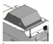
Top cover Shutting the opening on the top prevents coolant or chips splashing outside of the machine A hole for the mist collector is provided
