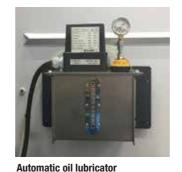
Regularly applies oil to all lubricating points on the tree axes.
