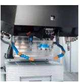
Column coolant nozzle Powerfully removes chips on and around the workpiece to prevent chips building up. \* Cannot be selected for the 40-tool magazine spec.
