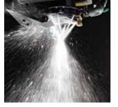
Tool washing, air-assisted type High discharge pressure and flow rate efficiently remove chips attached to the holder. Equipped with a filter clog warning function
