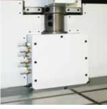
Hydraulic rotary joint (4 ports) Pneumatic relay box (12 ports) 12 pneumatic ports and 4 hydraulic ports have been prepared so that jigs that use pneumatic or hydraulic pressure can be mounted easily. \* For the R450Xd1, the Y-axis travel decreases when a hydraulic rotary joint is used.
