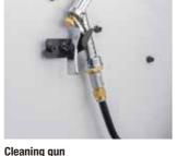
Helps clean the workpiece or chips inside the machine after machining.
