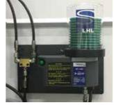
Automatic grease lubricator Regularly applies grease to all lubricating points on the three axes. \*Manual greasing is required for the standard specification model.
