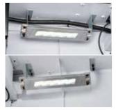
Work light (1 or 2 lamps) LED lamps are used to extend lamp life and save energy. \* For the R450Xd1, the 1st lamp is installed on the right side, and the 2nd lamp on the left side. For the R650Xd1, the 1st and 2nd lamps are both installed on the left side.
