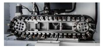
For the 40-tool magazine, the machining room is separated from the tool stocker by a shutter type door. This prevents chips entering the magazine.
