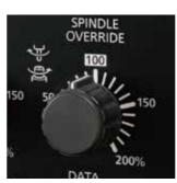
Spindle override Spindle speed can be changed without changing the program.
