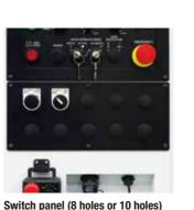
Various switches, such as automatic door open/close switches, are set in specific locations. The switch panel (8 holes) is also available so that the position of the manual pulse connector can be changed.
