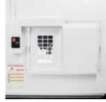
Side door with transparent window Makes setup or tool change from the side easier. The machining room can be checked through the window \* Standard for the R450Xd1 with 22/28-tool magazine and the R650Xd1.
