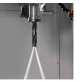
Coolant Through Spindle (CTS) Can be selected from 3.0 MPa or 7.0 MPa. Pump and tank are not included.
